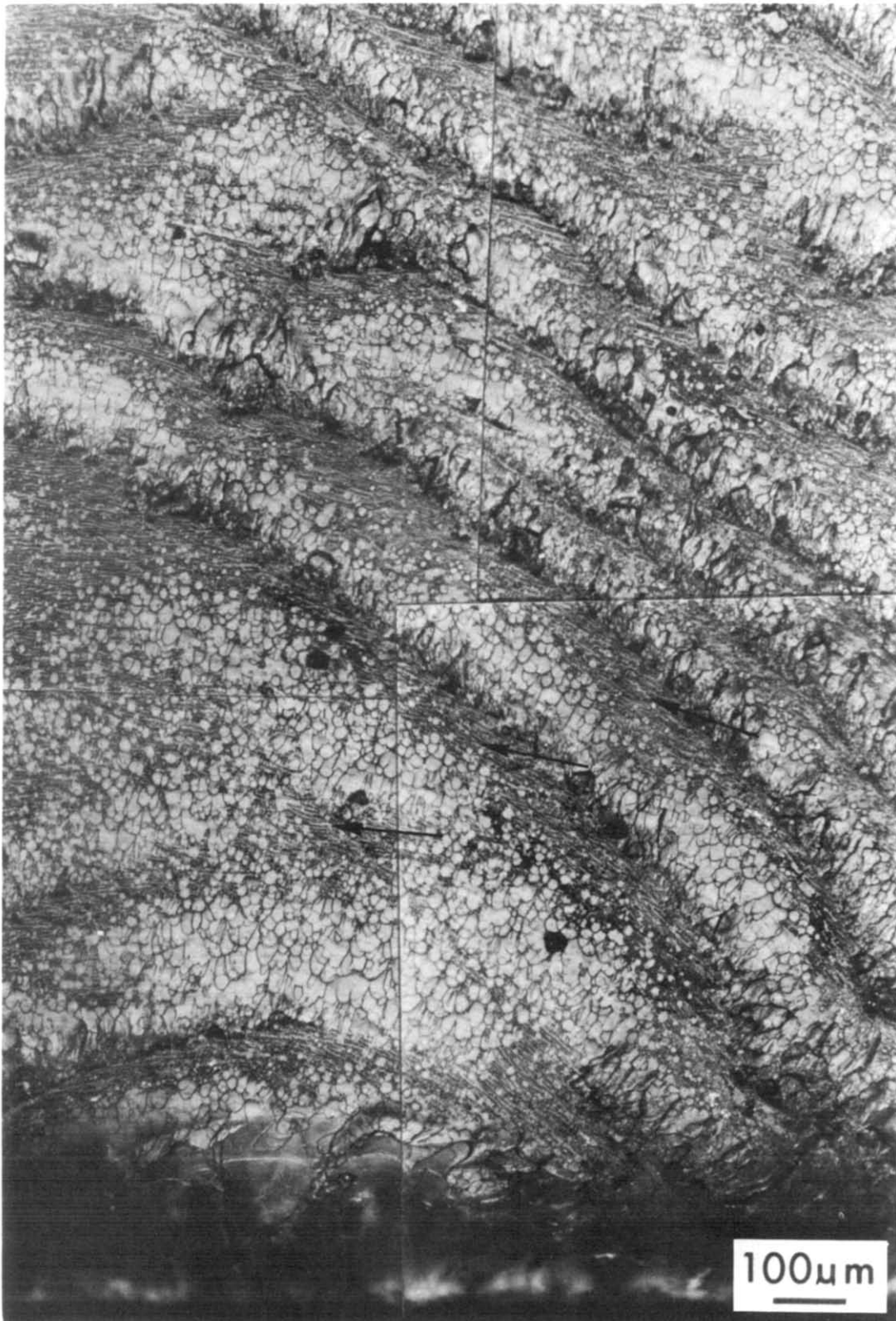
Figure 4 Arrays of linear fine features, in the mist (?) and hackle area (enlarged view of Figure 2, \bar{M}_v = 110\,000 ). Examples of these arrays are indicated by arrowheads. The nature of these features is unknown. Note also the intersecting bands of parabolas between the mirror region and the first full rib
